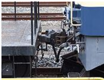
Two railway cars interlocked and joined together by a knuckle coupler
